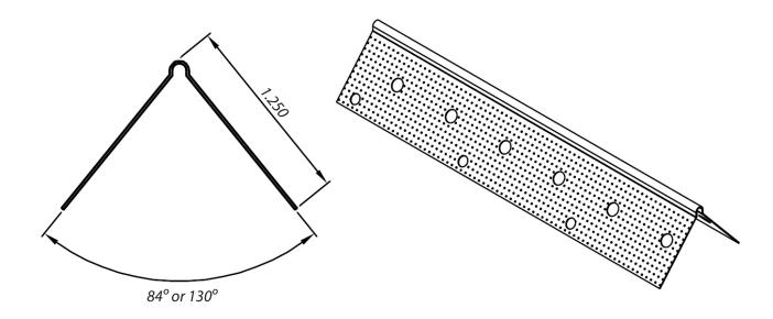
Our cornerbeads conform to Canadian steel standards. They are available in standard 7, 8, 9, 10 and 12 foot lengths (90 and 135 Deg).
