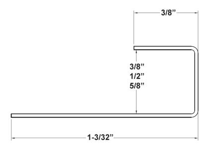
Our metal J trims conform to Canadian steel standards. They are available in standard 10' lengths in 3/8", 1/2" and 5/8" thicknesses. J trims serve to protect sides of gypsum panels around doors and windows or when gypsum panels rest on other materials.
