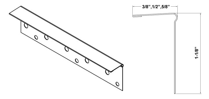
Our metal L trims conform to Canadian stel standards. They are available in standard 10' lengths with 3/8", 1/2" or 5/8" finished side. L Trims serve to protect sides of gypsum panels around doors and windows when no moulding is installed.
