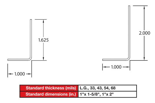
Our metal angles conform to Canadian steel standards. They are available in standard 10 foot lengths. They are available in the dimensions and thicknesses stated in the above table. You may also order dimensions, thicknesses and lengths that corespond to your project needs.
