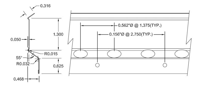
Our metallic resilient bars conform to Canadian steel standards. They are available in standard 12 foot lengths. They are an economical means of reducing noice transmission for wood or metal structual or load bearing partitions. Minimum coating for this product is G40.
