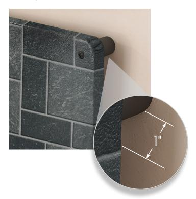
When using the stove board as a ceiling protector, a common minimum required distance from the top of the stove to the combustible ceiling is 48-in. This safety tip should be considered when installing a wood-burning stove in the basement of an older home, where the ceiling might be lower. An installer/user should always check the wood-burning stove appliance manual for additional safety reminders and instructions.
